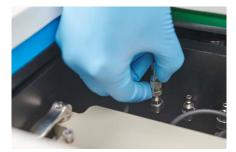
Figure 15. Removing the gassing lid out of the incubation chamber.
