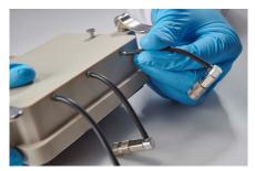
Figure 10. Attachment of the tubing to the gassing lid.
