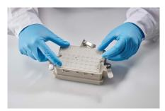
Figure 8. Preparation of the gassing lid E-BDR32 microfluidic experiments in the RoboLector XT instrument.
