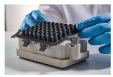
Figure 9. Attachment of the robotic lid to the gassing lid E-BDR32.
