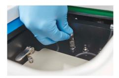
5. Attach the tubing of the gassing lid to the push-in connectors on the shaking table at the front side of the microbioreactor incubation chamber. Now, the cultivation experiment can start.
