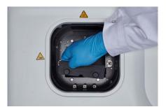
Figure 12. Placing the adapter plate into the 32-mode position.
