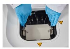
Figure 13. Placing the gassing lid into the incubation chamber.
