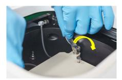
Figure 14. Push down the metal levers to fixate the gassing lid.
